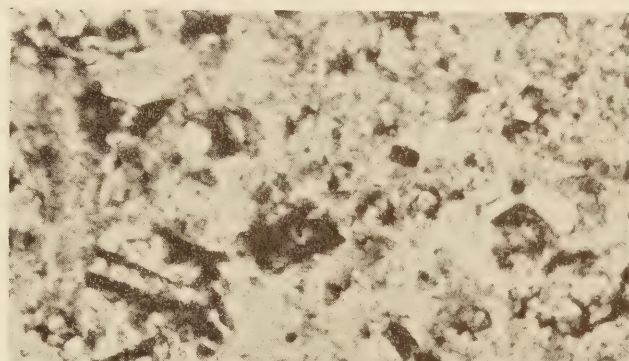
Neat cement cylinder stored 8 years in water
